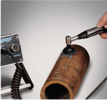
In-situ/Field metallography is widely used for microstructure analysis on large parts (samples) that cannot be easily carried or where destructive preparation is not permissible such as storage tanks, piping system, power plants, etc. In-situ Metallography allows for quick on-site evaluation of a component. There are numerous advantages in using in-situ/field metallography.
