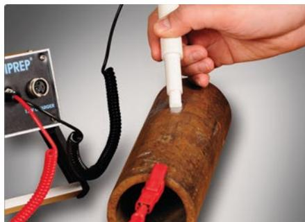
MOBIPREP With the Etching Pen for Electrolytic Etching
