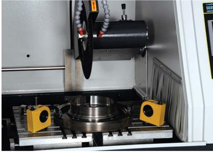
**SERVOCUT 501 is an advanced universal metallographic cutting machine used to cut a very wide range of materials.**
